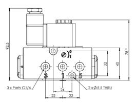
\* Minimum height with plug connector rotated through 90 degrees.
