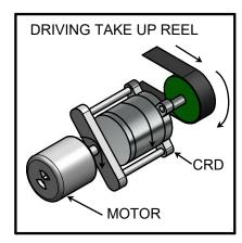
A CR dashpot can be used as a slipping drive between a geared motor and a take up reel for winding tape or wire on to a reel. If sized correctly the tension in the tape can be maintained within reasonable limits for a ratio of maximum to minimum reel radius of up to 2.5. Difficulty sometimes arises because it is necessary to select the correct motor speed as well as dashpot rate.
