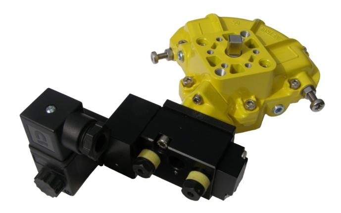
An option available on Kinetrol Models 03 to 15, the NAMUR interface allows for direct mounting of solenoid valves removing the need for external piping.
