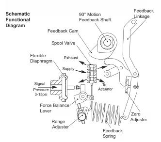
The AP positioner moves an actuator to a position set by a 3-15psi control signal and holds it there. Its features are:
