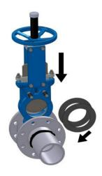
6. When the flanges have cooled down, insert the gate valve again with gaskets. The arrow on the body must coincide with the flow direction.
