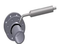
5. Weld the flanges to the piping.
