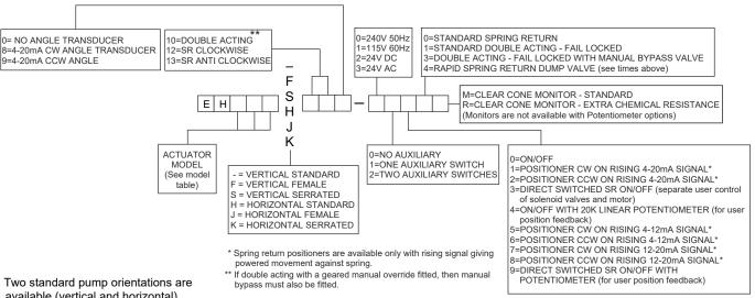
I wo standard pump orientations are available (vertical and horizontal). Consult Kinetrol if other arrangements are required. All units will be supplied with vertical axis actuators unless otherwise specified.
