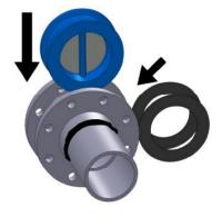
6. When the flanges have cooled down, insert the valve again with gaskets. The arrow on the body must coincide with the flow direction.
