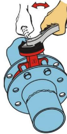
8. Open the valve orifice and ensure that the butterfly is easy to move.
