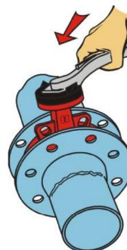
6. After the flanges have cooled down, insert the valve, and ensure sufficient clearance (see Fig. 1).
